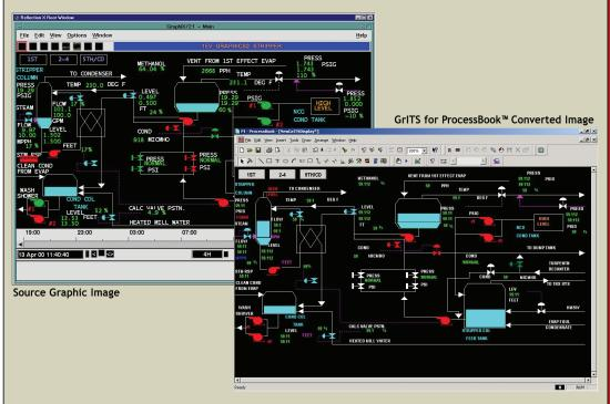
PI ProcessBook displays created with GrITS for ProcessBook can be saved as Displays in a PI ProcessBook, Independent Display Files (PDI files), Bitmaps, JPEG files, and SVG (Scalable Vector Graphics) files for use with RtWebParts.
